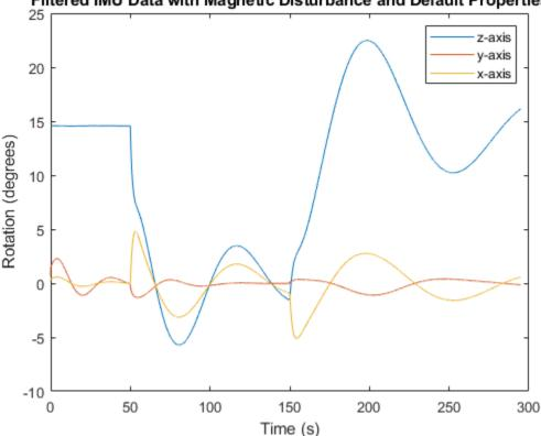
The magnetic jamming was misinterpreted by the AHRS filter, and the sensor body orientation was incorrectly estimated. You can compensate for jamming by increasing the MagneticDisturbanceNoise property. Increasing the MagneticDisturbanceNoise property increases the assumed noise range for magnetic disturbance, and the entire magnetometer signal is weighted less in the underlying fusion algorithm of ahrsfilter.
