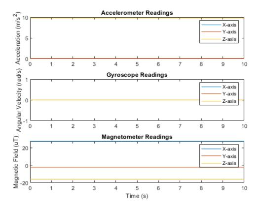
Orientation is not specified and the ground-truth motion is stationary, so the IMU sensor body coordinate system and the local NED coordinate system overlap for the entire simulation.
