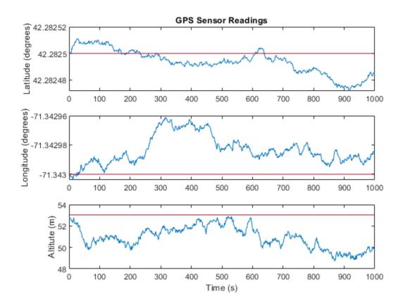
The position readings have noise controlled by HorizontalPositionAccuracy, VerticalPositionAccuracy, VelocityAccuracy, and DecayFactor. The DecayFactor property controls the drift in the noise model. By default, DecayFactor is set to 0.999, which approaches a random walk process. To observe the effect of the DecayFactor property:
