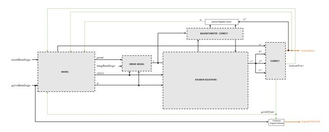
Before the first iteration, the accelReadings, gyroReadings, and magReadings inputs are chunked into DecimationFactor-by-3 frames. For each chunk, the algorithm uses the most current accelerometer and magnetometer readings corresponding to the chunk of gyroscope readings.
