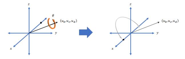
The quaternion representation of the rotation may be expressed as  $q = \cos(\theta/2) + \sin(\theta/2)(u_b i + u_c j + u_d k)$ , where  $\theta$  is the angle of rotation and  $[u_b, u_c, and u_d]$  is the axis of rotation.
