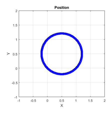
The trajectory output now appears circular. This is because the waypointTrajectory System object $^{\text{\tiny TM}}$  minimizes the acceleration and angular velocity when interpolating, which results in smoother, more realistic motions in most scenarios.
