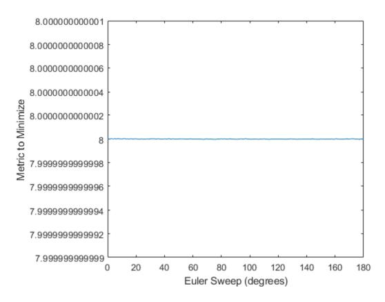
Quaternion means are usually calculated for rotations that are close to each other, which makes the edge case shown in this example unlikely in real-world applications. To average two quaternions that are significantly far apart, use the slerp function. Repeat the experiment using slerp and verify that the quaternion mean returned is more intuitive for large distances.
