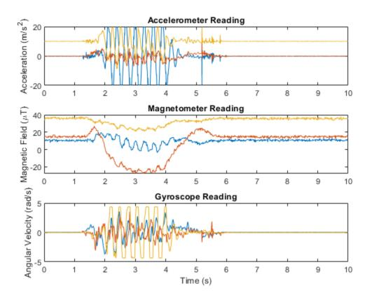
Create an ahrsfilter and then fuse the IMU data to determine orientation. The orientation is returned as a vector of quaternions; convert the quaternions to Euler angles in degrees. Visualize the orientation of the sensor body over time by plotting the Euler angles required, at each time step, to rotate the global coordinate system to the sensor body coordinate system.
