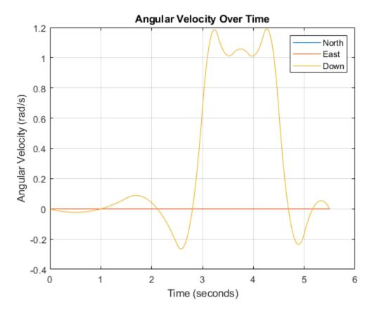
Note that while the generated trajectory now fits within the spatial boundaries, the acceleration and angular velocity of the trajectory are somewhat erratic. This is due to over-specifying waypoints.
