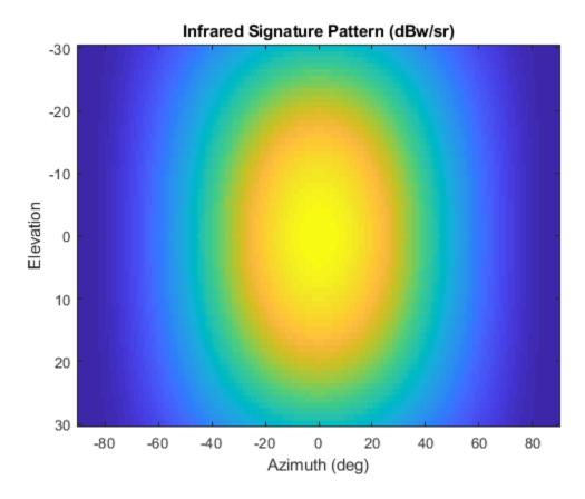
Get the IR intensity value at 25 degrees azimuth and 10 degrees elevation. value(irsig,25,10)
