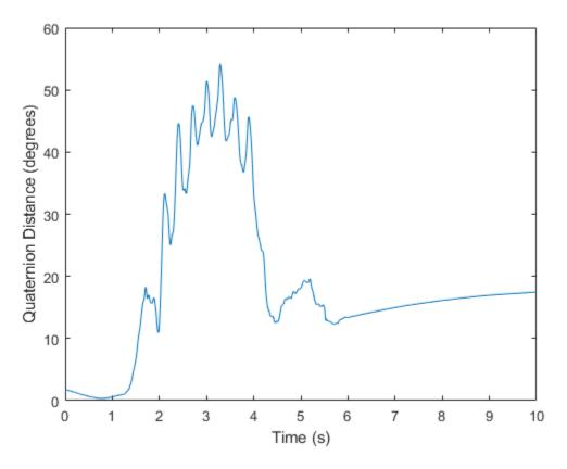
Modify the default ahrsfilter properties so that the filter converges to gravity more quickly. Increase the GyroscopeDriftNoise to 1e-2 and decrease the LinearAccelerationNoise to 1e-4. This instructs the ahrsfilter algorithm to
