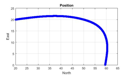
Inspect the orientation, velocity, acceleration, and angular velocity over time. The waypointTrajectory System object<sup>TM</sup> creates a path through the specified constraints that minimized acceleration and angular velocity.
