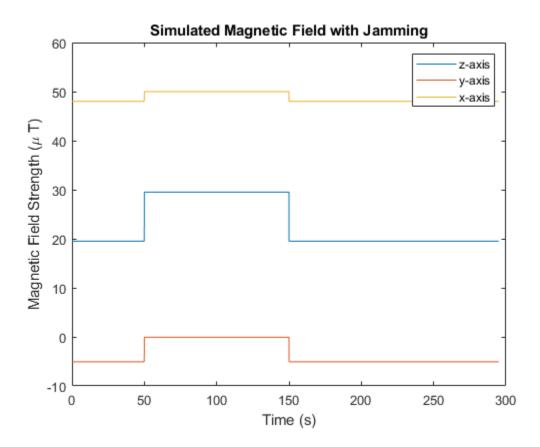
Run the simulation again using the magReadings with magnetic jamming. Plot the results and note the decreased performance in orientation estimation.
