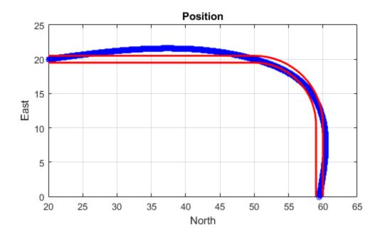
To create a trajectory within the bounds, add additional waypoints. Create a new waypointTrajectory System object $^{\text{TM}}$ , and then call it in a loop to plot the generated trajectory. Cache the orientation, velocity, acceleration, and angular velocity output from the trajectory object.
