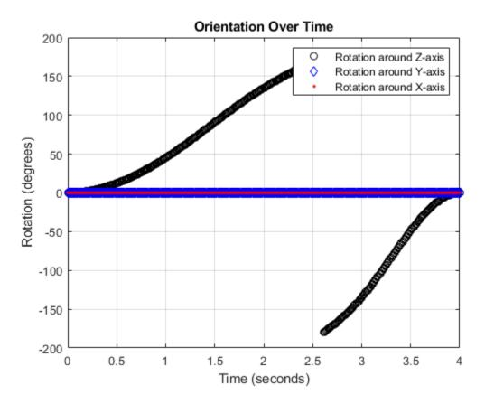
The waypointTrajectory algorithm interpolates the waypoints to create a smooth trajectory. To return to the square trajectory, provide more waypoints, especially around sharp changes. To track corresponding times, waypoints, and orientation, specify all the trajectory info in a single matrix.
