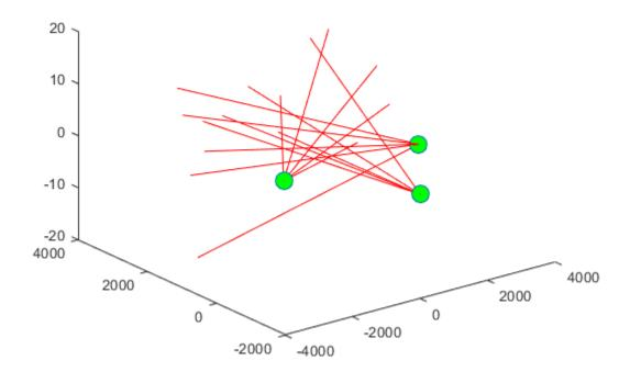
Create a  ${\tt staticDetectionFuser}$  to fuse angle-only detections using the measurement fusion function  ${\tt triangulateLOS}$ .
