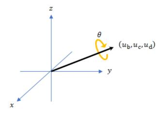
Given a quaternion in the form, q = a + bi + cj + dk, where a is the real part, you can solve for  $\theta_a$ :  $\theta_a = 2\cos^{-1}(a)$ .
