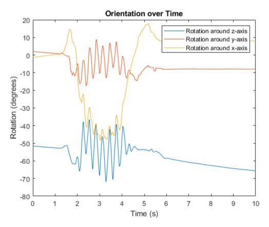
In the IMU recording, the shaking stops after approximately six seconds. Determine the resting orientation so that you can characterize how fast the ahrsfilter converges.
