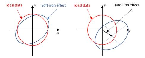
The underlying algorithm in magcal determines the best-fit ellipsoid to the raw sensor readings and attempts to "invert" the ellipsoid to produce a sphere. The goal is to generate a correction matrix A to account for the soft-iron effect and a vector b to account for the hard-iron effect. The three output options, 'eye', 'diag' and 'sym' correspond to three parameter-solving algorithms, and the 'auto' option chooses among these three options to give the best fit.
