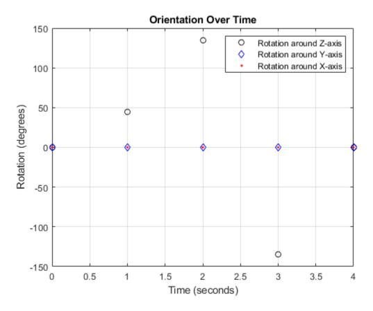
So far, the trajectory object has only output the waypoints that were specified during construction. To interpolate between waypoints, increase the sample rate to a rate faster than the time of arrivals of the waypoints. Set the trajectory sample rate to 100 Hz and call reset.
