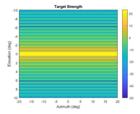
Create a tsSignature object and plot an elevation cut at 30° azimuth.
