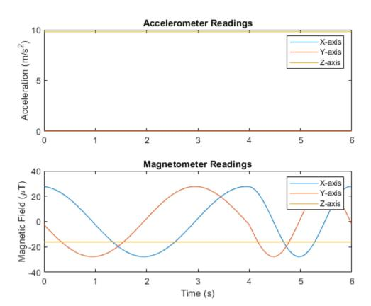
The accelerometer readings indicate that the platform has no translation. The magnetometer readings indicate that the platform is rotating around the *z*-axis.
