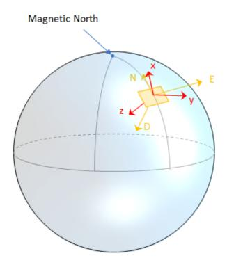
Recall that orientation of a sensor body is defined as the rotation operator (rotation matrix or quaternion) required to rotate a quantity from a parent (NED) frame to a child (sensor body) frame:
