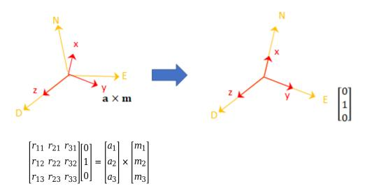
The second column of the rotation matrix corresponds to the cross product of the accelerometer reading and the magnetometer reading:
