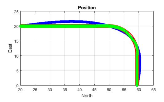
The generated trajectory now fits within the specified boundaries. Visualize the orientation, velocity, acceleration, and angular velocity of the generated trajectory.
