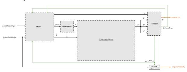
Before the first iteration, the accelReadings and gyroReadings inputs are chunked into 1-by-3 frames and DecimationFactor-by-3 frames, respectively. The algorithm uses the most current accelerometer readings corresponding to the chunk of gyroscope readings.
